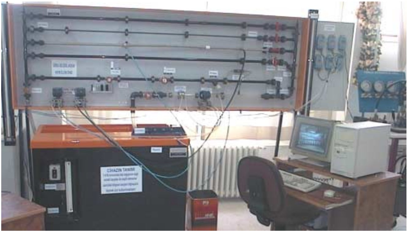
Figure 1: Picture of a fluid friction apparatus and a data acquisition system.
